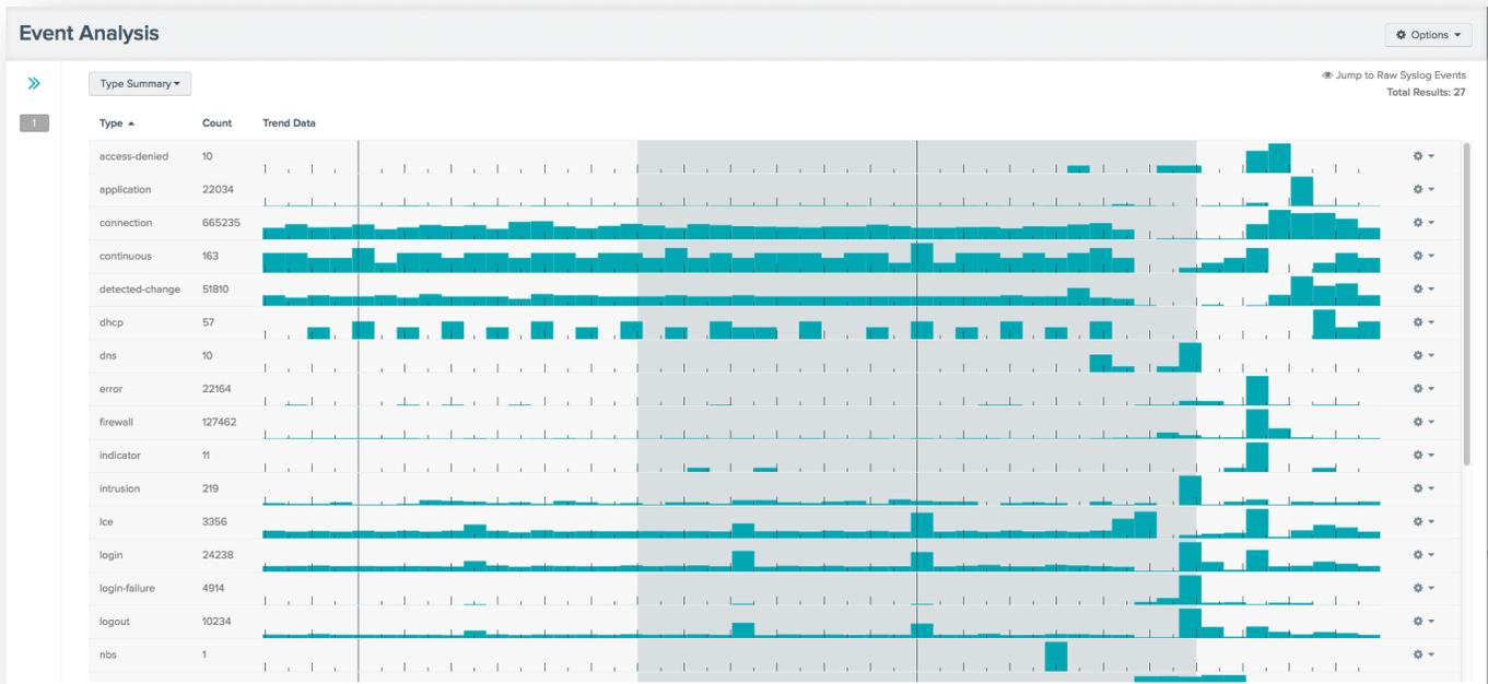
This portion of events (the screen image only shows “access-denied” types through “intrusion” types for 24 hours) offers some interesting patterns. The dark areas represent 6:00 PM through 6:00 AM. The activity graph shows that some types of events occur all the time, such as the “intrusion” types and “error” types. If a SecurityCenter user were to mouse over the graphs, they would be shown a pop up image of the total amount of events at that point and the exact times.
